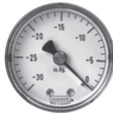
Y —Vacuum Gauge mounted in porting head P/N LFT-363
